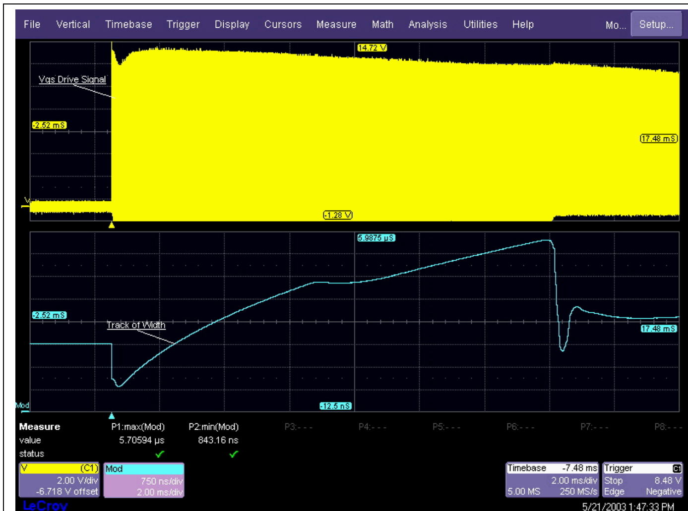
Figure 2 A study showing the startup of the power supply
